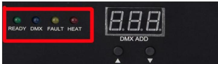
**READY:** Green light when the "READY" green light turns from flashing into light on, it indicates that the machine is ready to work.
