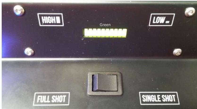
The green bar represents the capacity of the battery in the gun. When fully charged the Bar will be completely green. When the battery is depleted only the first led on the bar will flash red.
