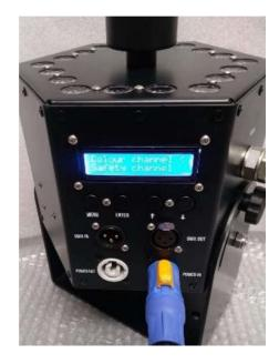
Connect the DMX cable to the DMX in connector. Connect the other end of the DMX cable to the DMX Controller.
